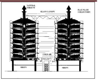
Fig.5 Ventilation at East Gate Center, Harare
