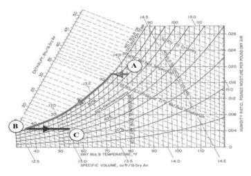
Fig.14 Conventional Cooling and Dehumidification Process in Psychrometric Chart
