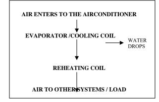
Fig.13 Scheme in Conventional Air Conditioners
