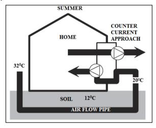
Fig.9 Experimental Configuration by Pierre et al [12]
