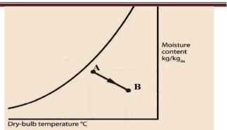
Fig.15 Desiccant based Dehumidification
