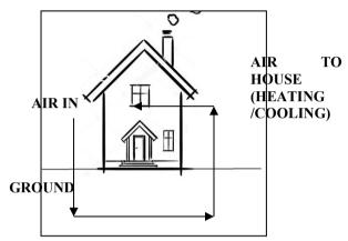
Fig.8 Simple Configuration of Ground Heat Exchangers for HVAC
